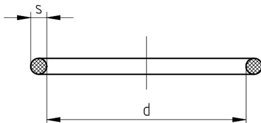
OR per pistoni in due pezzi      O-Ring for piston in two pieces
