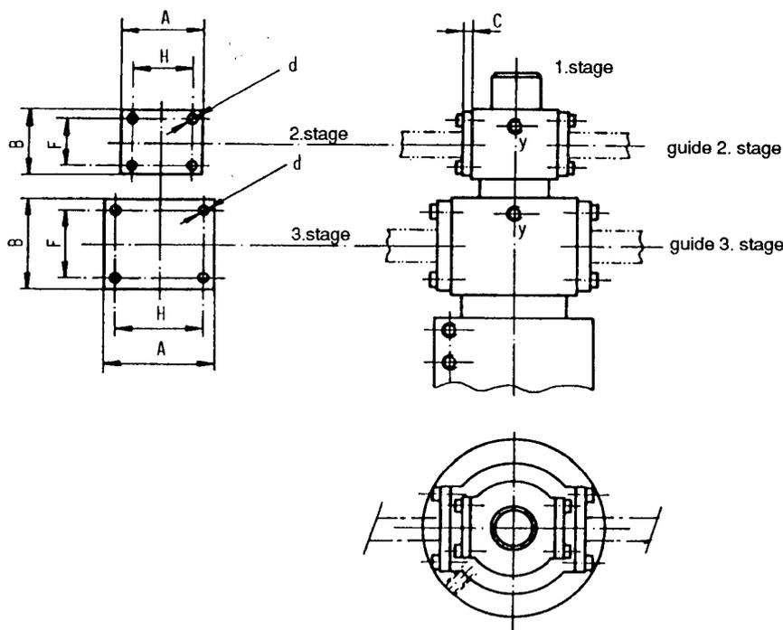
Screws for Yoke Plates : M 8 x 25 for d = 10
