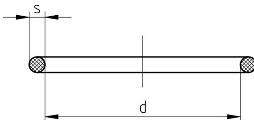
OR per cilindri in due pezzi      O-Ring for piston in two pieces
