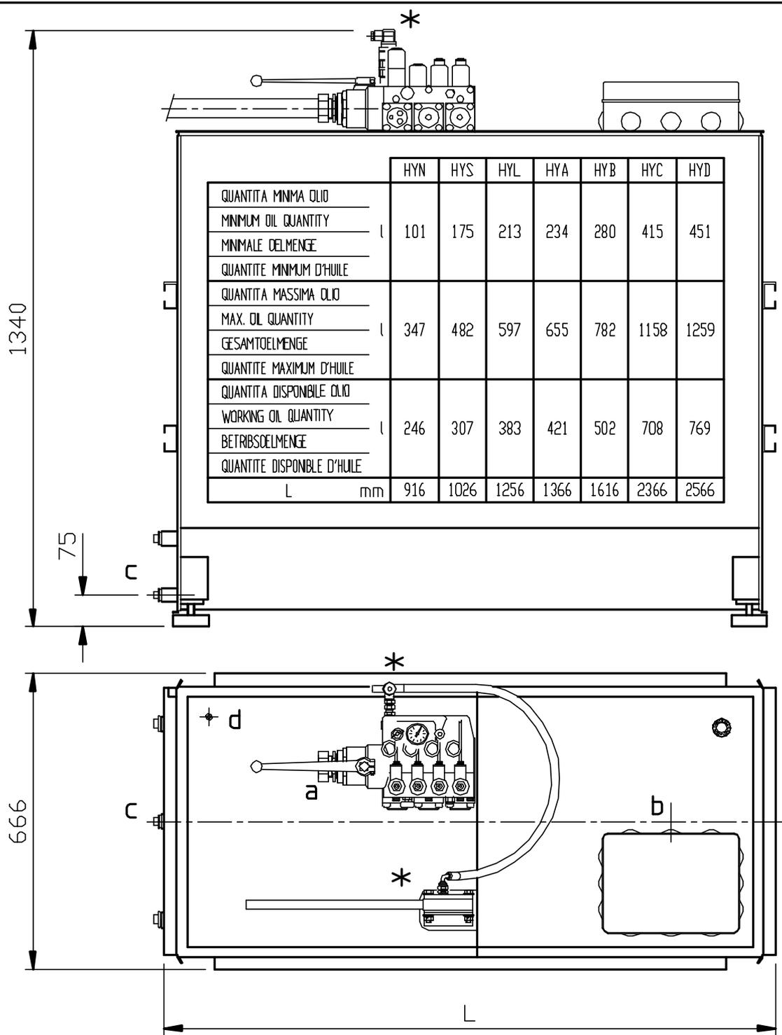
\* POMPA A MANO E PRESSOSTATO SOLO SE RICHIESTI O NECESSARI / MANUAL PUMP AND PRESSURE SWITCH AS OPTIONAL OR IF REQUIRED
