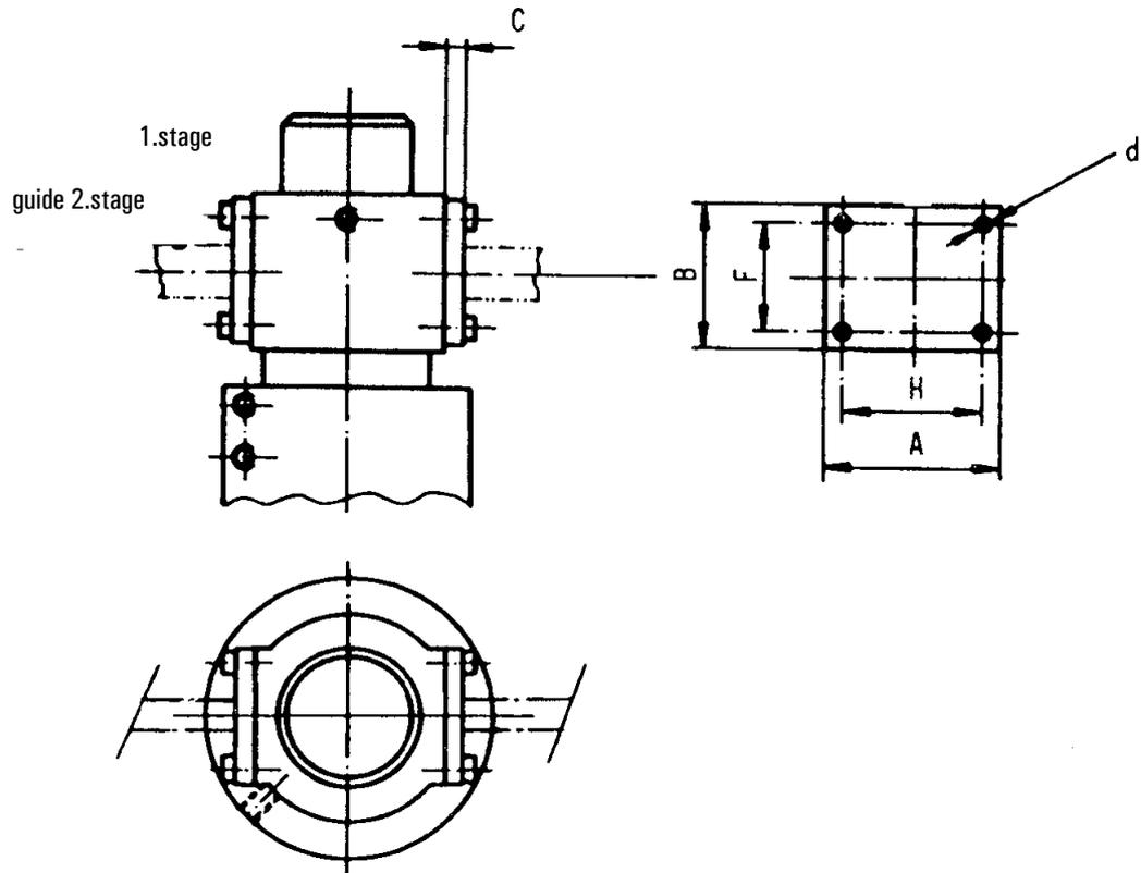
Screws for Yoke Plates :    M 8 x 25 for d = 10
